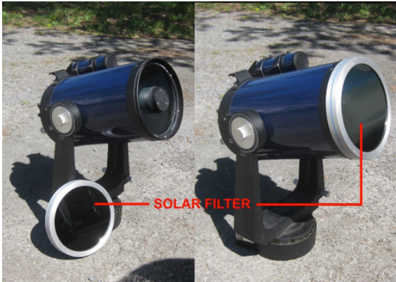
A full-aperture filter for solar observing.
